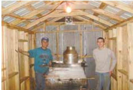
Paul and Mark Collins cook maple tree sap in a portable cooker that eliminates the need to transport sap out of the woods.
