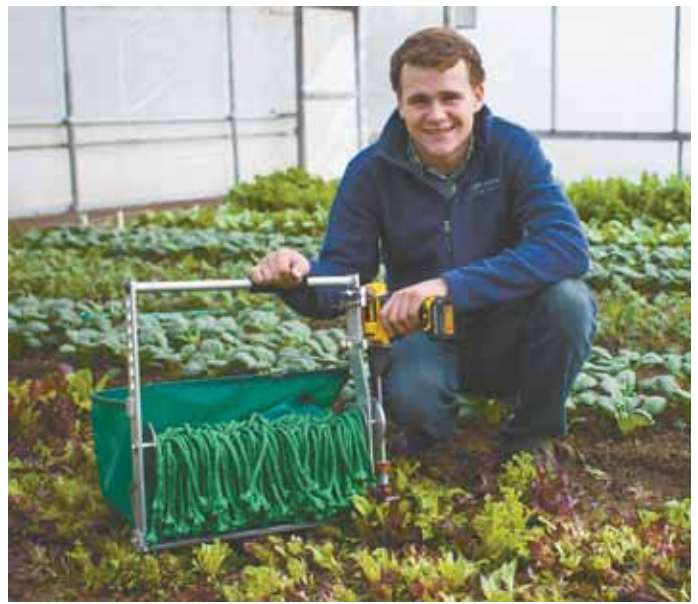
Jonathan Dysinger with his Quick Cut Greens Harvester. It uses a 14-in. dia. brush with tassel-like tips to push the greens across a cutting edge and into basket.
