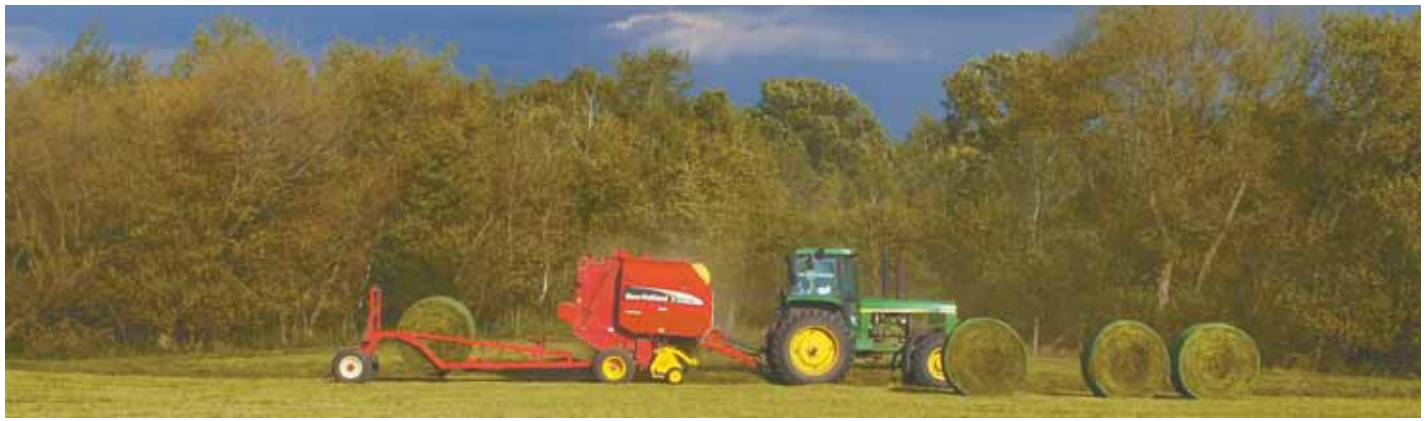
Thanks to rear swivel wheels, the Bale Positioning System follows directly behind baler, catching two big bales as they're ejected from baler.
