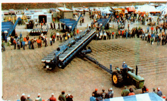
In less than three minutes, the planter hydraulically pivots into the transport position.
