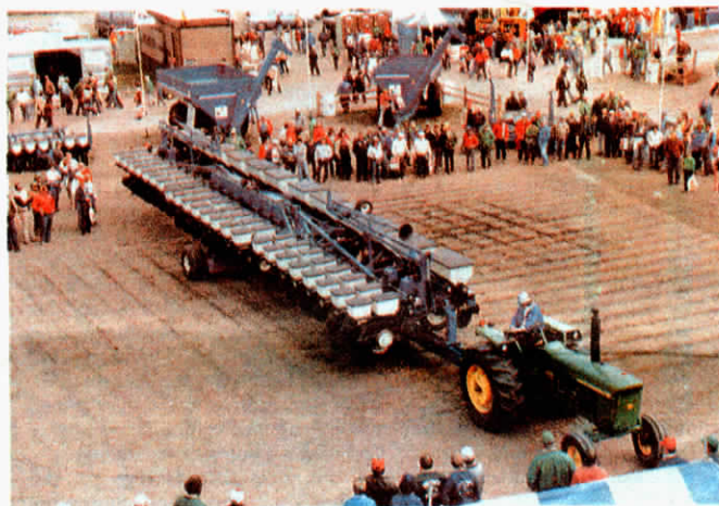
The 24-row planter has a 16½ ft. transport width.
