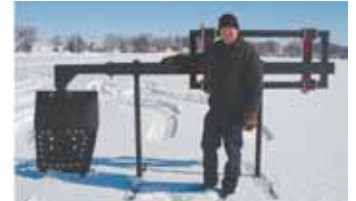
Jeff Frederick built this loader-mounted feed bunk plow to quickly clean out dirty feed and snow.
