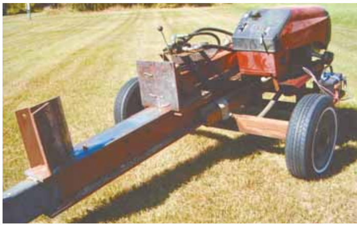
Mark Adelman and his son cut a 14 hp Murray garden tractor down to the engine, hood and dash to build this low-cost splitter.
