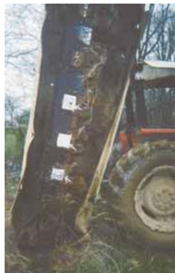
Metal wear plates under disc mower are marked in white.
