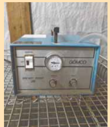
Criger installed a regulator on breast pump to control vacuum pressure.
