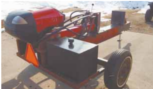
Back end of splitter rides on the axle and wheels off an old grain elevator.
