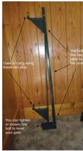
Gate leveling bracket bolts onto existing gate post. Lets you “relevel” a gate when it begins to sag.
