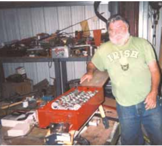
Jim Dolan’s aluminum can crusher bolts onto the table of an electric-operated log splitter. It flattens 20 cans at a time.
