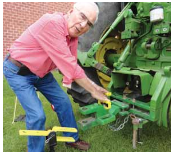
Harold Fratzke developed this telescoping, quick coupler tractor drawbar. “It takes the guesswork out of hooking up to any implement,” he says.
