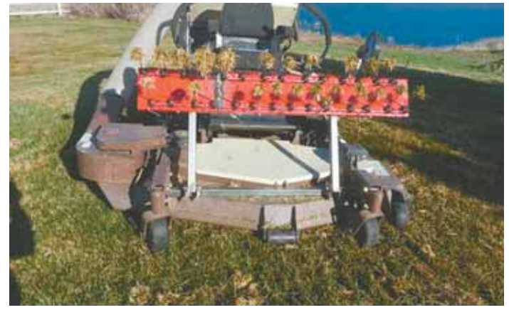
Hinged metal arms on dethatcher frame pivot on brackets bolted to mower deck, allowing Steffen to lift dethatcher for transport.
