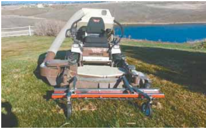
Matthew Steffen used a pair of new Sears pull-type dethatchers to build a front-mount dethatcher for his Grasshopper zero turn riding mower.
