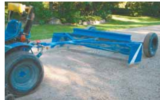
"We use it to maintain a 1/4-mile stretch of road in a high traffic area. It works like a little land leveler," says Marlin Galde, who built this 8-ft. wide, 3-pt. mounted box scraper.
