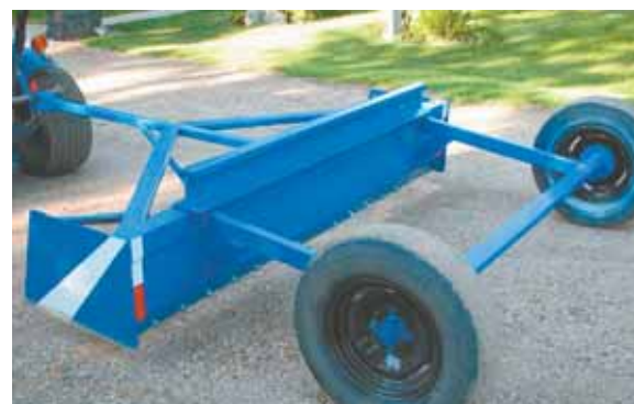
Box scraper is 8 ft. wide and rides on 15-in. rear flotation tires that extend 3 ft. back from the blade.
