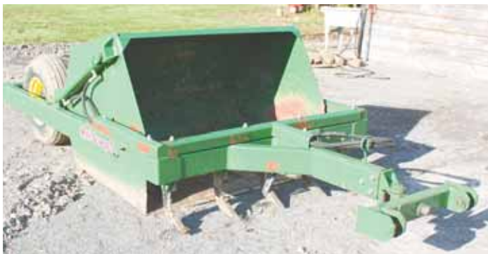
Dave Odom's homemade dirt scoop works just like big rigs you see on road crews. It mounts to a Cat. I or II tractor quick hitch.
