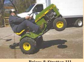
Schwab replaced the 11 hp engine on a Deere 111 with a 20 hp V-twin Briggs & Stratton, adding wheelie bars on back.
