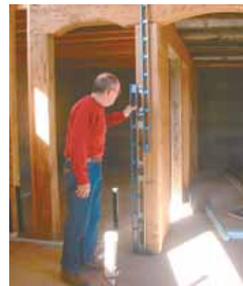
The 5-ft. 3-in. Plumbit level extends out up to 13 ft. 10 in. You can use it to level everything from foundations to doorways.
