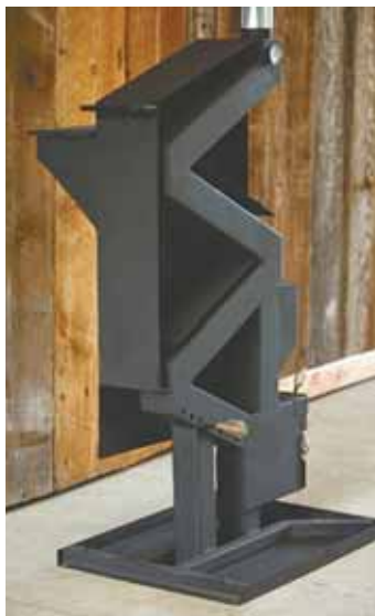
Stove runs on gravity feed. Pellets flow into a primary burn basket, then into a secondary burn chamber where they finish burning. Ashes fall into a tray below.
