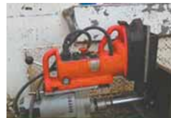
Boring tool connects to a Milwaukee magnetic drill to re-size worn holes in tractor bolsters.
