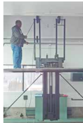
Two wheels on the top of lift push ceiling door open to make room for 6 1/2 by 10-ft. platform.
