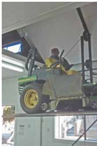
Two wheels on the top of lift push ceiling door open to make room for 6 1/2 by 10-ft. platform.
