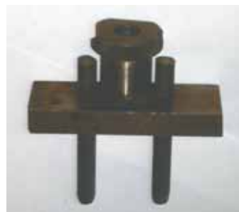
Carl Schafer came up with this simple jig for repairing seed boots on Deere 750 no-till drills. It eliminates the need to remove the seed boots and use a drill press.
