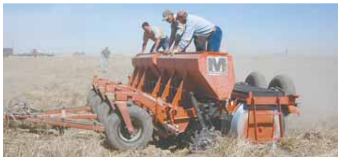
Taller packer wheels with higher axles help prevent residue from building up and plugging the drill.
