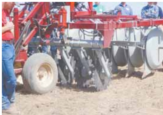
Big wheel drills are designed to help plant into high-residue fallow ground, say researchers at Washington State University and product developers at The McGregor Co.
