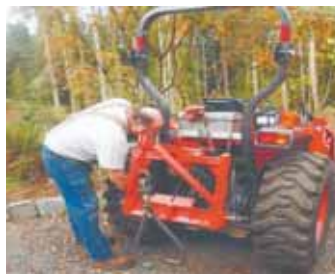
Dave Boriack uses a 34 hp Kubota 4-WD tractor to pull his home-built, 3-pt. mounted log skidder. It's fitted with a hook and a pair of log tongs.
