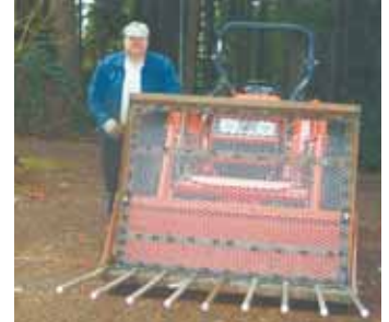
Bucket-mounted brush rake is made from expanded metal welded to an angle iron frame.
