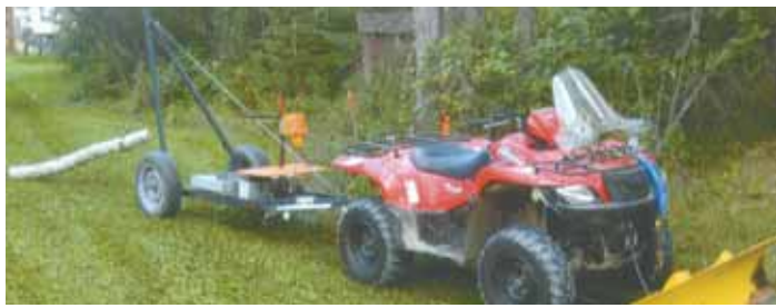
Gerald Thorsen pulls this home-built log skidder behind his Honda 450 ATV. Skidder's 7-ft. high hinged boom raises and lowers the log.
