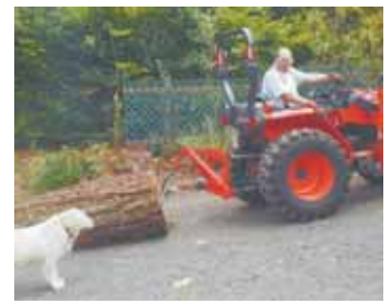
Dave Boriack uses a 34 hp Kubota 4-WD tractor to pull his home-built, 3-pt. mounted log skidder. It's fitted with a hook and a pair of log tongs.
