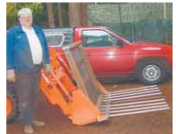
A series of 42-in. long steel forks are spaced 6 in. apart at bottom of rake.
