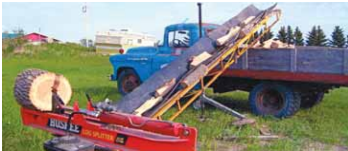
Tilman Jones converted a small square hay bale elevator into this 16-ft. long firewood conveyor. A V-shaped rubber funnel keeps the wood in contact with the chain.
