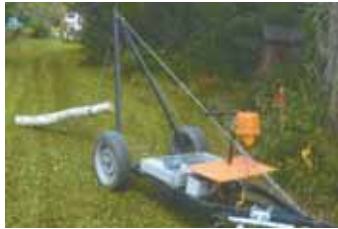
Cable attached to top of boom manually adjusts boom angle.
