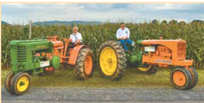
By splitting a 1939 Allis Chalmers WC and a 1949 Deere B and then putting the halves together, Dotterer and Grieb made what they call Half-Rite, Half-Rong tractors.
