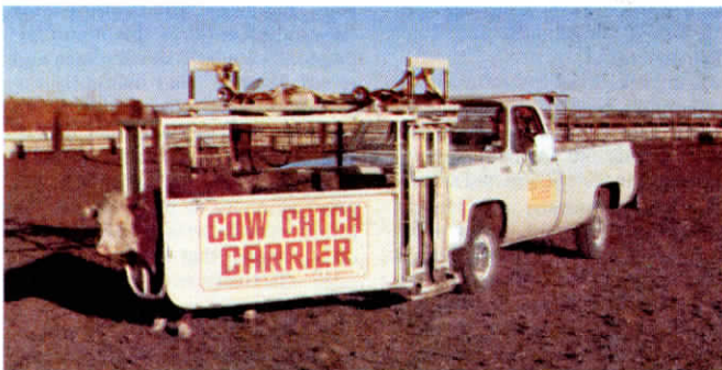
As pickup overtakes animal, driver operates folding gates to gradually ease it into the chute.
