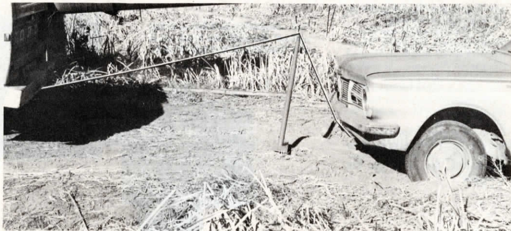
Lift-Out is set at about 45° angle. As towing vehicle (or winch) moves forward, the device helps lift the stuck vehicle as it's being pulled out.
