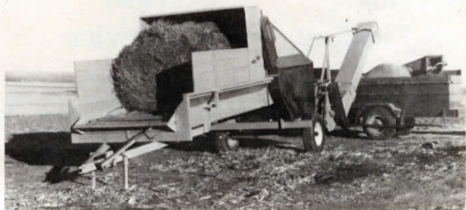
Elevator shown with this model is optional. The bed, equipped with a variable speed apron, is only 42 in. high and large enough to accommodate two of the largest big bales.
