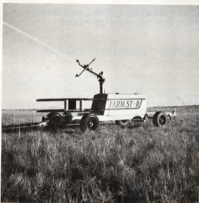
Cable buildup on a drum controls the drive ratio to provide constant ground travel speed.
