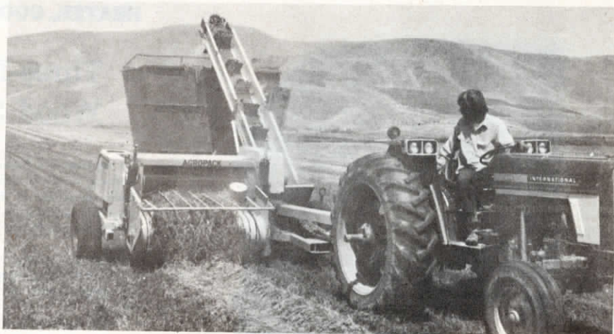
The Agropack mini-roll machine has a throughput capacity of about 6 to 8 tons per hour. Mini-rolls it makes are 5 to 7 in. in dia., and 4 to 7 in. long.
