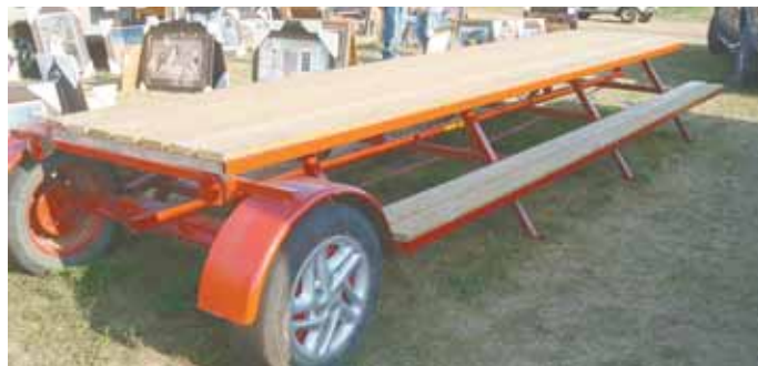
Portable 18-ft. long picnic table rides on the chassis from an old van and hooks up to pickup's receiver hitch. Inventor Robert Hanselman rents the table for $50 a day.
