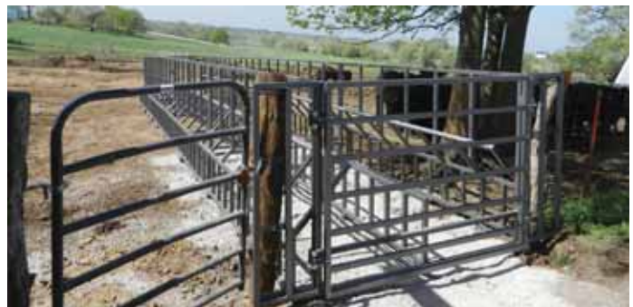
EZ Load hay feeder is made up of modules that bolt together. Bales are loaded onto a central rail that's elevated off the ground to keep hay dry.
