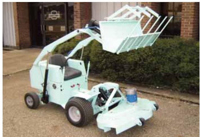
Electric-powered garden tractor can be equipped with a loader. Front-mount 3-pt. hitch can be used to support a 42-in. mower deck fitted with an electric motor.
