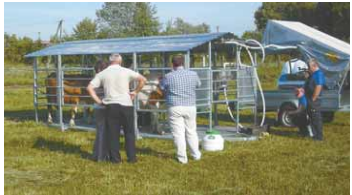
Lithuanian milking system “brings the milking parlor to cows rather than have the cows come to the parlor. Cows don’t waste energy walking to a parlor.”
