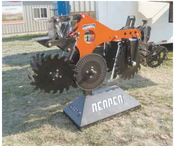
Free-floating row cleaner uses two large 22-in. sawtooth coulters that remove virtually all the trash in front of the shank, without throwing it over into the next row.
