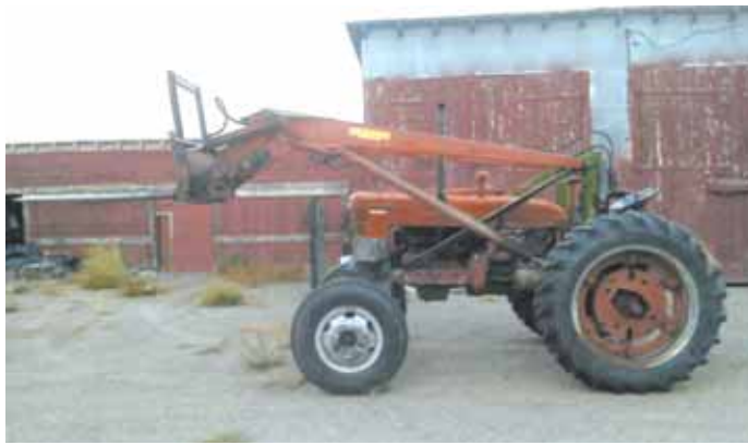
The front end of this Farmall tractor couldn't handle the weight of big round bales, so the Careys equipped it with an axle off a 1979 Ford 1 1/2-ton pickup.
