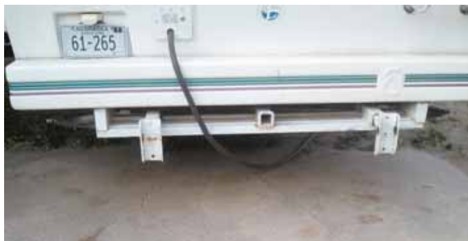
Hitch arms on trailer pin to brackets on either side of receiver hitch to securely hold front of trailer.
