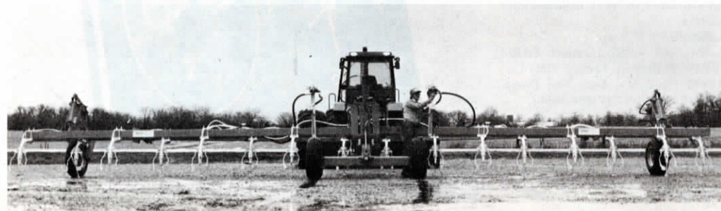
In transport position, rear-folded toolbar applicator is lower than height of the tractor. The 45 ft. wide unit folds to narrow, 15 ft. width.
