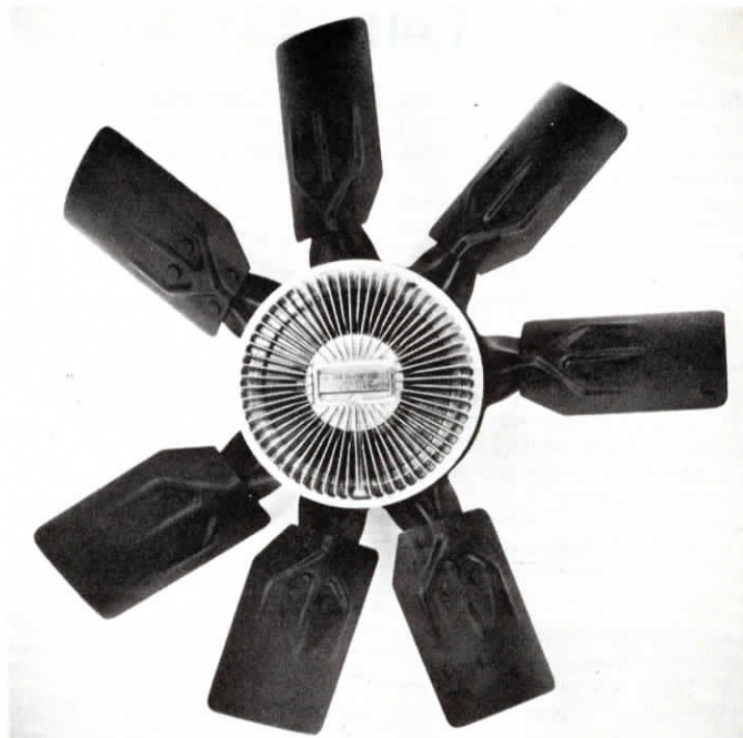
Operation of the Duro Drive viscous fan clutch is similar to that of any automatic transmission. The clutch is a fluid coupling, controlled by a thermal unit which is sensitive to the temperature of air flowing from the radiator core.
