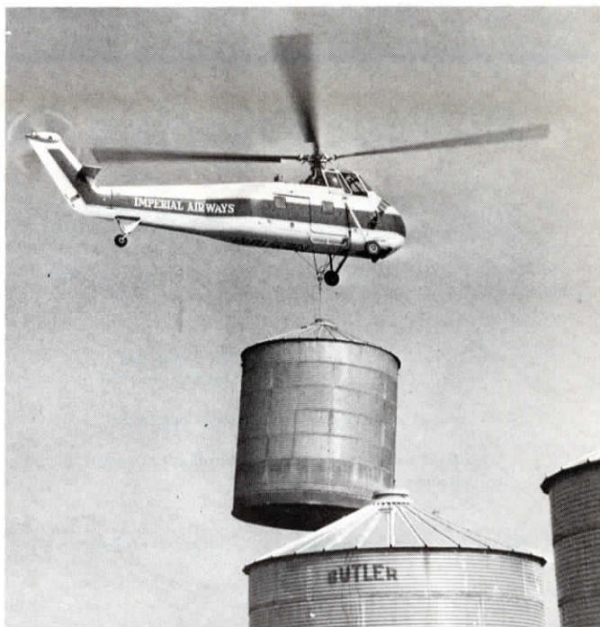
Imperial Helicopter's fleet of 10 helicopters, operating in 10 different states, are often called upon to move grain bins and other items weighing up to about 10 tons.
