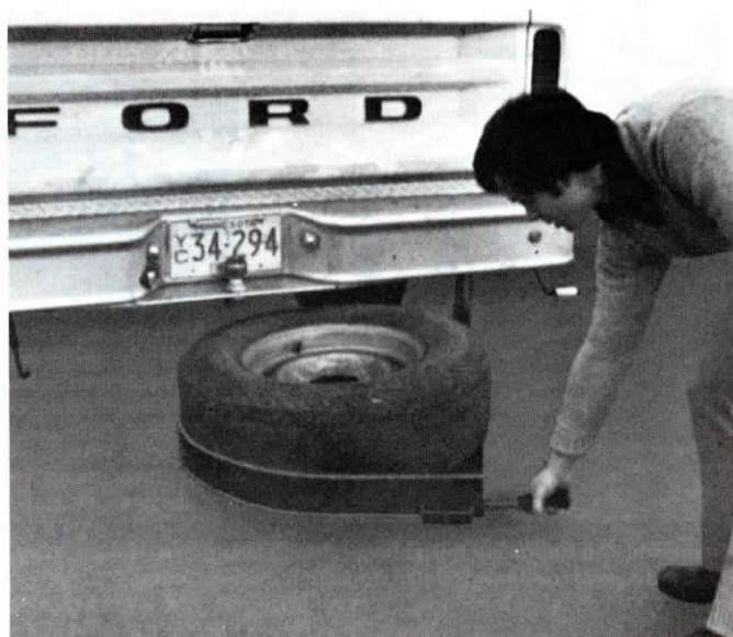
Redi-Carrier cranks down and swings out from under the pickup, eliminating the need for crawling or kneeling to retrieve the spare tire.
