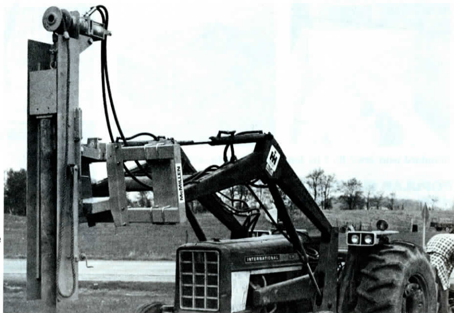
Self-dumping Rotamixer turns counter-clockwise to discharge mixed load.
