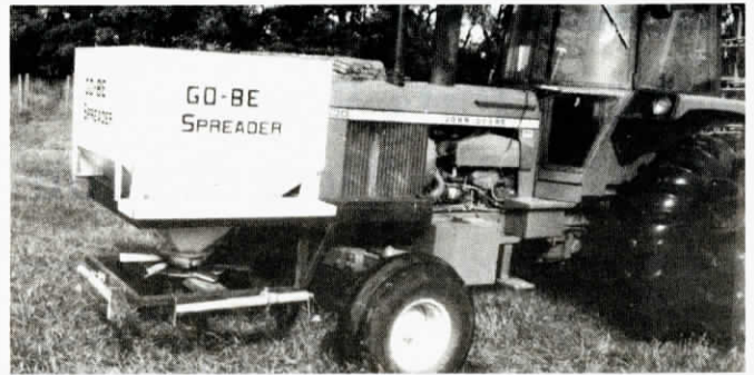
Seeding width is adjustable to match width of your pull-behind cultivator, chisel plow, harrow or other tillage equipment.
