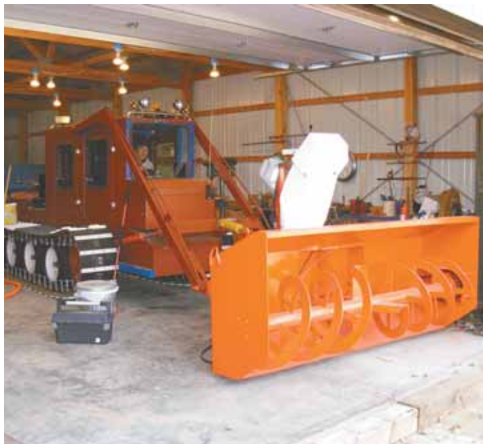
Track-mounted snow mover is equipped with a dozer blade and a blower that'll grind through 5-ft. drifts.
