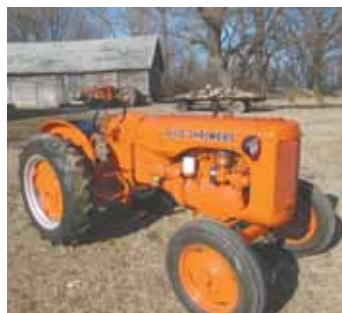
Jim Willette lowered the profile on his Allis Chalmers "B", making the tractor easier to get on and off.
