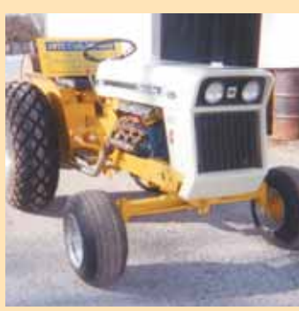
Mervin Jones repowered his Cub Lo-Boy with a Cobra 302 engine out of a Ford Mustang. The 200 hp, V-8 engine fit almost perfectly.
