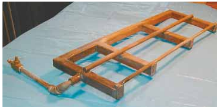
Homemade grate was made by welding up some 1-in. sq. tubing, then drilling 1/8-in. dia. holes into the tubing and adding an air hose fitting to one end.
