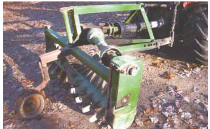
“It works good for doing landscaping work and for establishing lawns,” says Gerald Johnston, who built this 3-pt. mounted, pto-operated machine that doubles as a rototiller.
