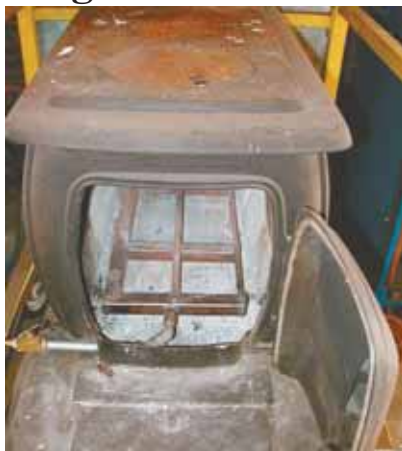
To start the fire, the operator connects an air compressor hose and opens the valve enough to force air under the fire.
