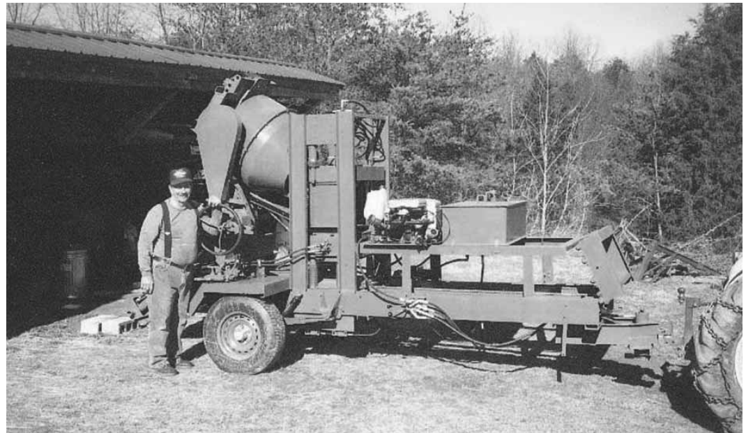
"It lets anyone make high quality blocks right on the job site, and works fast," says Chester Fisher, about the portable cement block making machine he made to help Haitians rebuild their schools and churches.
