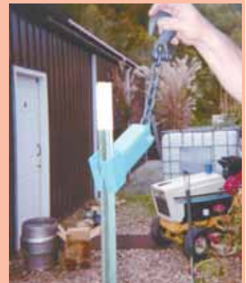
"No slip" T-post puller lets Ricky Plunkett use a loader bucket or bumper jack to pull posts out of the ground without slipping.
