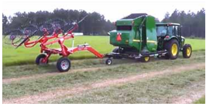
The Hay Train attaches to the baler tongue, allowing you to tow the rake in-line behind the baler on the road and off to the side in the field.
