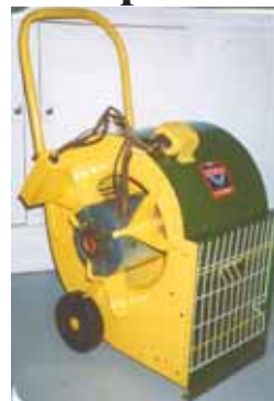
Galen Reichart converted an old furnace blower into this shop fan that runs off any 110-volt outlet.
