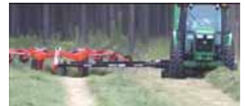
Unit is designed to pull 8, 10 and 12-wheel ground-driven rakes.
