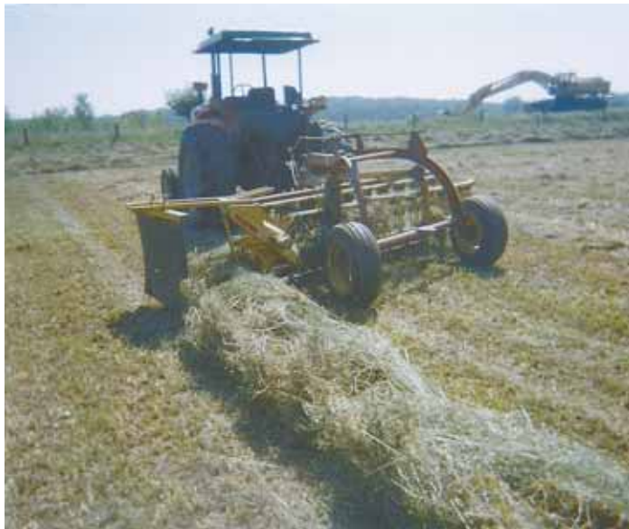
Harold and Dale Scherer found that adding a baffle to the end of their power rake helps form perfect windrows, even when raking at high speeds.
