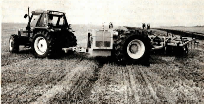
Tillage tools attach directly to the 110 hp. turbo-charged tow behind "Yoke" power unit which lets a small to medium-sized tractor do the work of a big 4-WD.
