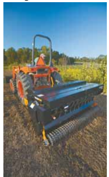
Woods seeder can plant 3 different crops at a time, all at different depths.
