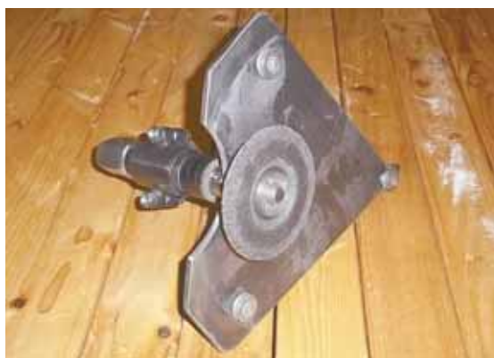
Vince Osburn made this grinding tool to fit inside the differential housing on his Deere 2020 tractor, allowing him to resurface the brake contact area.
