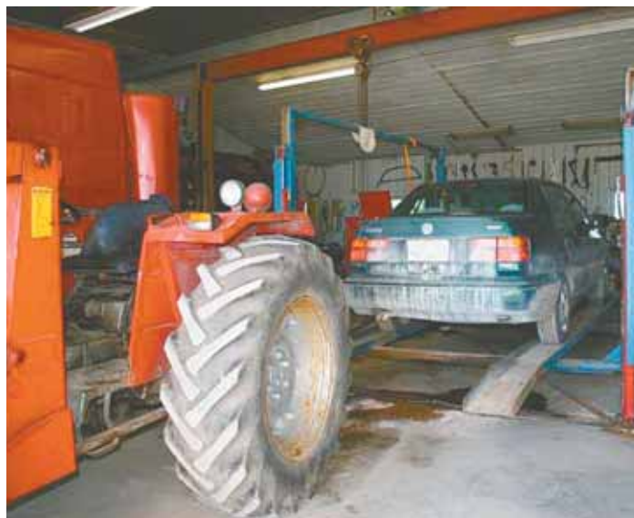
Portable hydraulic car and truck hoist has two 12-in. wide, channel iron wheel ramps that are raised and lowered on 4 lifting posts.
