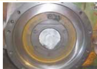
Photo at left shows grinding tool being used to resurface brake; photo at right shows resurfaced brake installed in differential housing.
