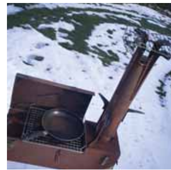
“Toolbox” wood stove has a chimney and metal rack “pot warmer” at one end. Both the legs and part of the chimney come off and store inside toolbox for easy transport.
