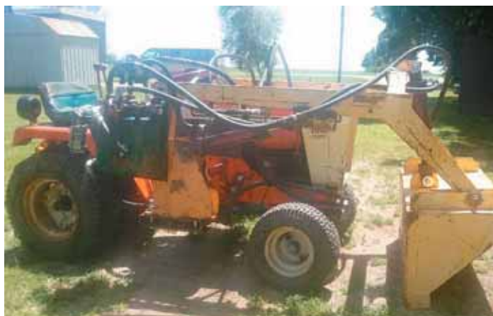
Kevin Nell built this front-end loader for his Simplicity garden tractor. A pto-driven pump on front of tractor is used to raise and lower the bucket and also to tilt it.
