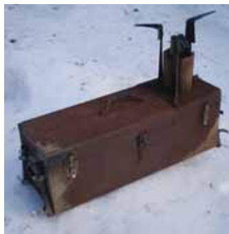
“Toolbox” wood stove has a chimney and metal rack “pot warmer” at one end. Both the legs and part of the chimney come off and store inside toolbox for easy transport.
