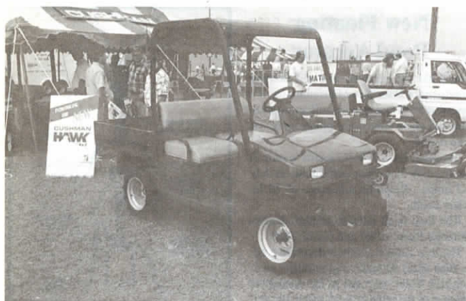
Cushman's new "Hawk" features oscillating chassis and lugged tires that allow it to ride smoothly over even the roughest terrain.
