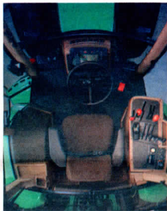
New "cab-forward" design allowed engineers to design larger cab with 40 percent more room. Note relocated vents around instrument console.
