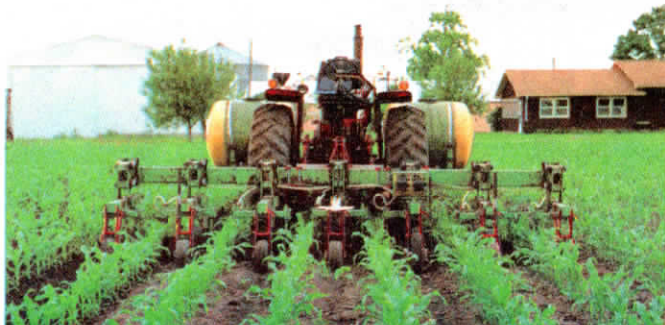
Danny Guy mounted new Glencoe 6-row cultivator on back of tractor and reversed the controls. Home-built 3-pt. quick hitch attaches cultivator rigidly to tractor.
