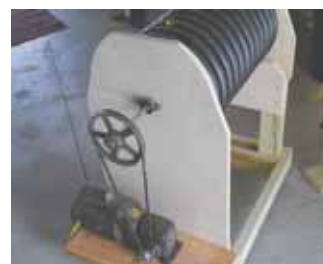
Dehulling drum was made from a length of 12-in. dia. plastic drain pipe.
