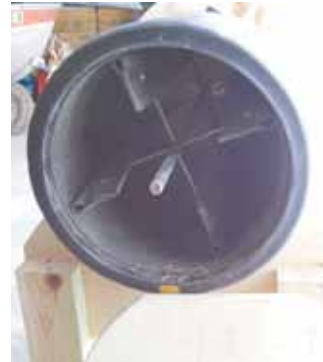
Tom Hohl made it easier to process wild rice by building his own dehuller. It uses a small electric motor to turn a fan-like mechanism inside a 2-ft. long drum.
