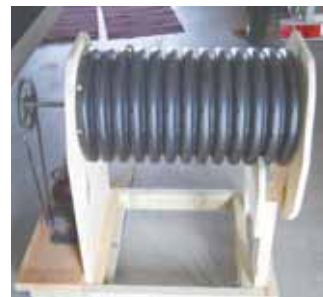
Tom Hohl made it easier to process wild rice by building his own dehuller. It uses a small electric motor to turn a fan-like mechanism inside a 2-ft. long drum.
