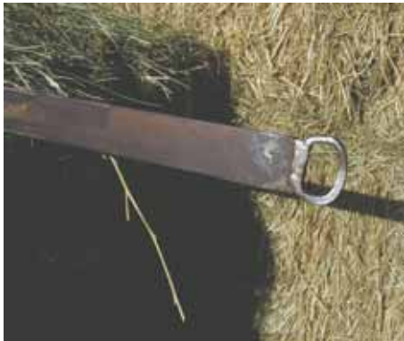
The eye of the "needle" holds the straps which keep the half-size bales together.
