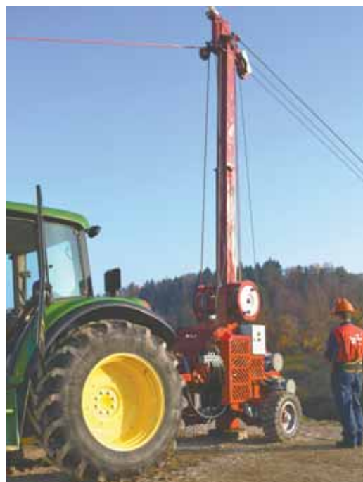
Pto-driven winch tower works like a ski lift to pull logs out of the woods.
