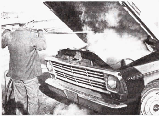
Exhaust from the engine serves as an air compressor which siphons fluid through a special nozzle.
