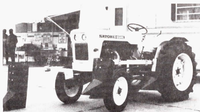
Crop dividers are designed to separate tall, bushy and viny crops by pushing them to either side of the front or rear tractor tires.
