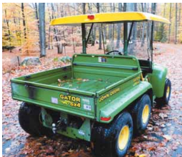
Joe Rishel built a cover for his Deere Gator out of an old fiberglass pickup topper. Metal struts from a camper awning support it.
