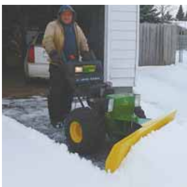
Don Campbell cut the auger and impeller off an old snowblower and replaced it with a 51-in. wide snow blade. "It'll push right through 6 in. of light snow," he says.
