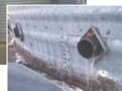
Ben Casper's Sectional Drying System uses fans to push fresh air through specially vented bins to dry the crop. No heat is needed. As air passes into the grain it picks up moisture that flows into exhaust tubes (right) that exit through the bin's sides.
