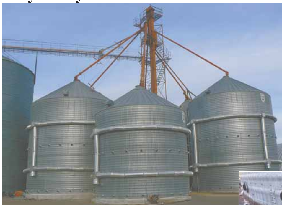
Ben Casper's Sectional Drying System uses fans to push fresh air through specially vented bins to dry the crop. No heat is needed. As air passes into the grain it picks up moisture that flows into exhaust tubes (right) that exit through the bin's sides.
