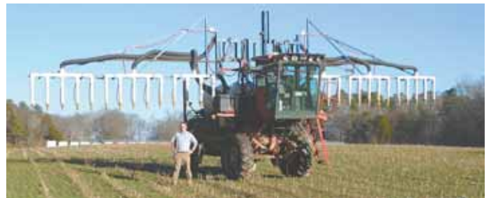
He assembled back and side booms, then mounted 35 specialty spray nozzles on them. Boom sections can be shut off individually.
