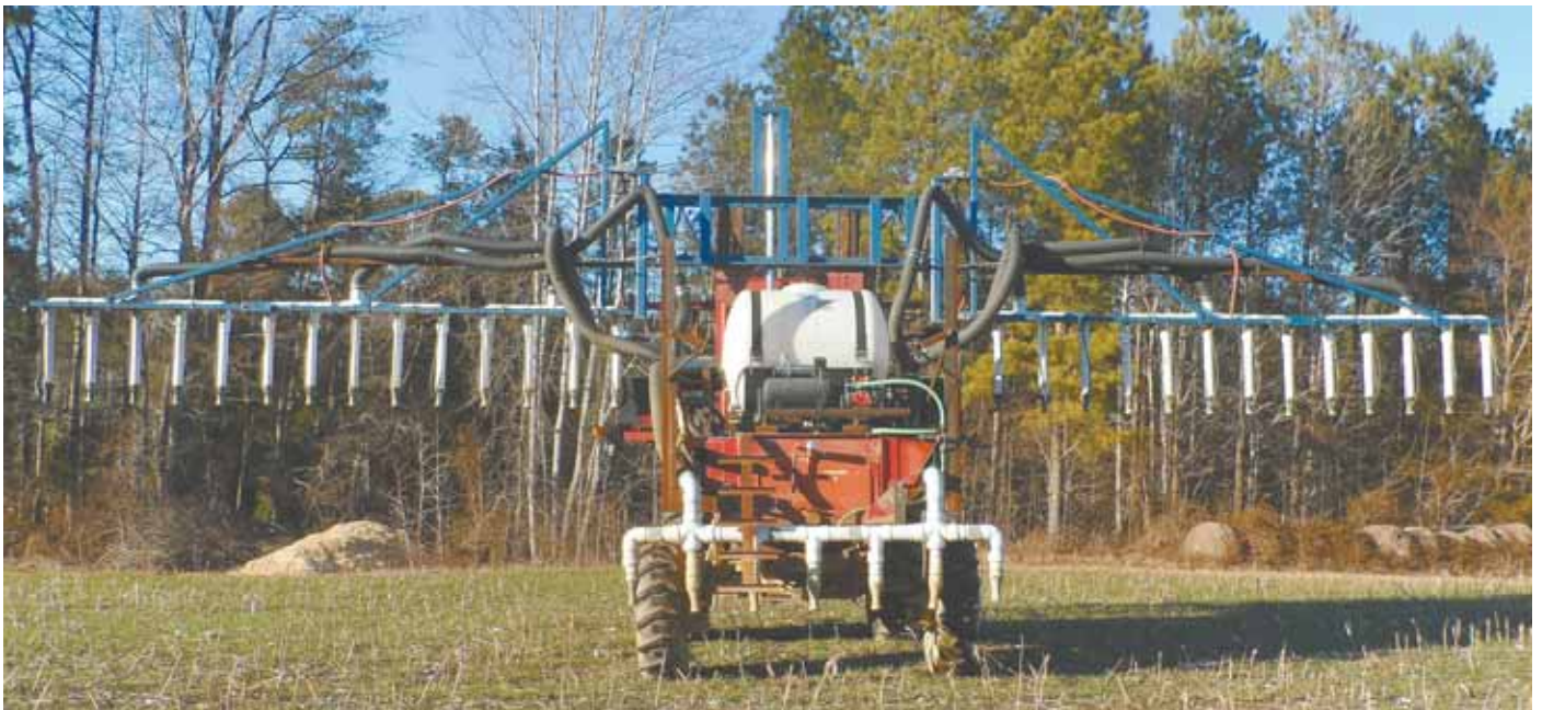
Peter Wilson converted an old Case IH 4-row cotton picker into a multi-section "air boom" sprayer for his vegetable and strawberry crops. The air system that previously moved cotton lint to the cargo basket now creates a high pressure fog that penetrates the canopy across a 48-ft. swath.
