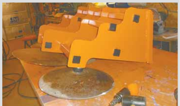
Dave Julian came up with a way to use recycled tillage disc blades as ice scrapers. Blades attach to loader arms.
