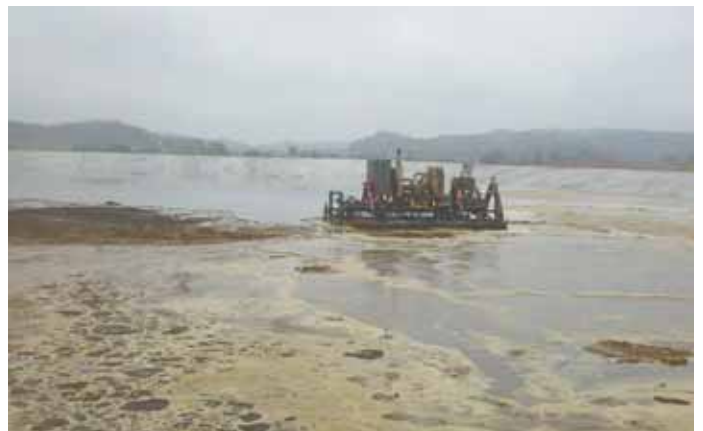
"It has better pressure control and handling features than other units on the market, and can stir up an 8 million gal. pit in only 8 hours," says inventor Chris Lindstrom.
