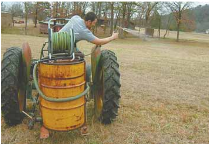
Allen Kimball can fight grass and brush fires right from his Deere 430's tractor seat using water from a 3-pt. hitch-mounted, 55-gal. barrel. It's filled and emptied by a side-mounted water pump.
