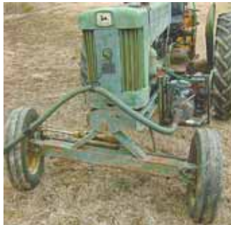
A 2-in. dia. hose on front of tractor pulls water from ponds or streams to fill barrel.
