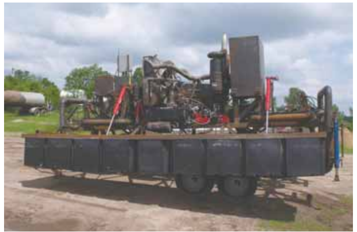
Manure agitation boat measures 10 ft. wide, 20 ft. long and weighs 14,000 lbs. It uses a powerful hydrostatic transmission system mated to 2 Italian-made Veneroni pumps.
