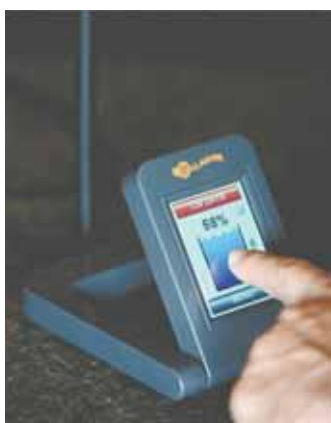
System uses a sensor to measure water pressure in tank. Information from the sensor is transmitted via solar-powered wireless communication unit (above) mounted on top of tank, to a desktop touchscreen display unit located up to 2 1/2 miles away.
