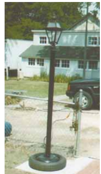
Leonard Seltzer used a spare tire and a length of muffler pipe to make this portable yardlight.
