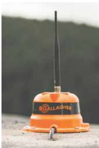
System uses a sensor to measure water pressure in tank. Information from the sensor is transmitted via solar-powered wireless communication unit (above) mounted on top of tank, to a desktop touchscreen display unit located up to 2 1/2 miles away.
