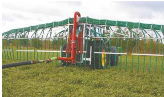
Cadman dribble bar is designed to apply liquid manure to standing crops. It can be used on any crop that can be sidedressed, including corn at early stages.
