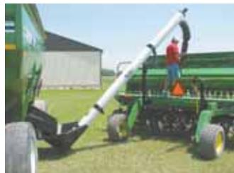
The 8-in. dia. Deere drill-fill auger bolts onto drill's rear frame. It rides parallel to the seed box for transport.
