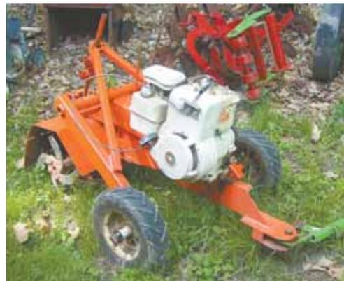
To convert rear tine tiller to a tow-behind model, Russ Wing replaced the tiller's self-propelled wheels and added an offset hitch.
