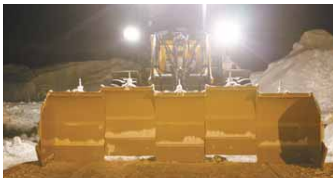
Snowblade is equipped with individual 2-ft. wide sections, which trip and then slide up and over uneven surfaces on-the-go.
