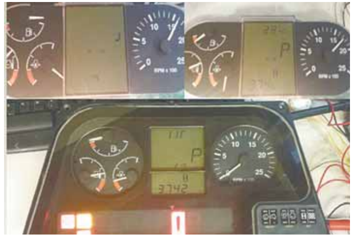
Before (top 2 photos) and after (bottom photo) repair of White 8510 tractor gauges. Gauges would sometimes not work or missing pixels would appear on the display.
