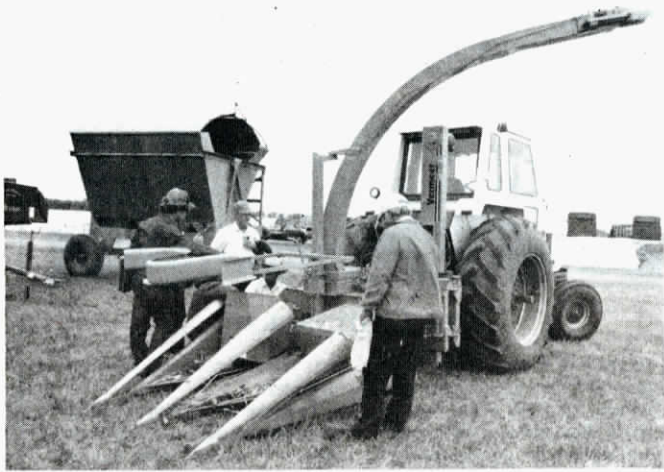
Chopper, shown in "reverse" position, features new energy efficient flywheel design.
