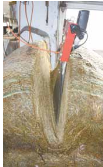
Electric-operated bale saw slices open big round bales with practically no effort.
