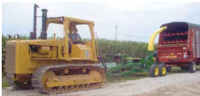
Michael Zimmerman modified his 1981 Caterpillar D5BSA crawler tractor to power pto-operated equipment, such as this 3-row silage chopper.
